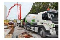
The two concrete hybrid trucks are equipped with electrical rotators that are fueled by the fossil free diesel HVO100. The rotator is charged by a generator when the engine is running and one charge drives the rotator for four hours. Besides less emissions it also contributes to a better work environment with less exhaust and noise.
